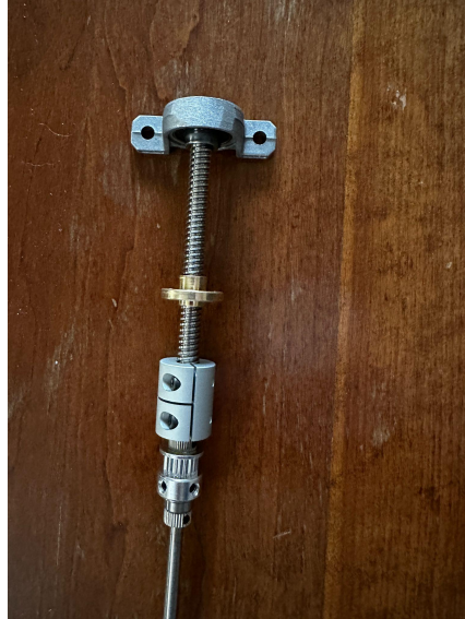
Figure 69; Threaded rod with pulley assembly
